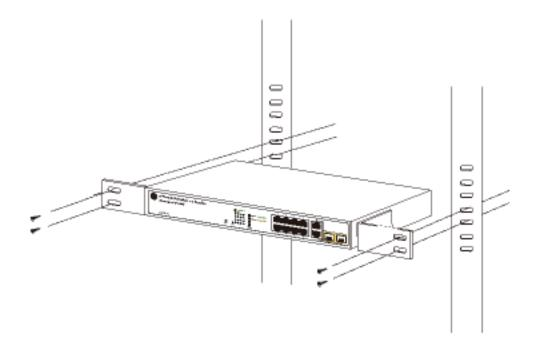
**Step 6:** Follow steps 4 and 5 of the Desktop Installation section to connect the network cabling and supply power to the Managed Switch.
